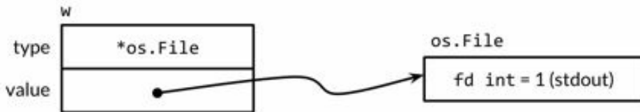
Figure 7.2. An interface value containing an *os.File pointer.
