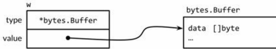
Figure 7.3. An interface value containing a *bytes.Buffer pointer.
